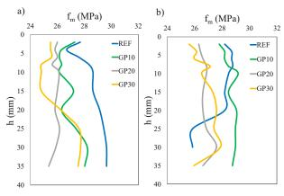
Fig.6 Calculated Compressive strength relative to sample height for mortar:
