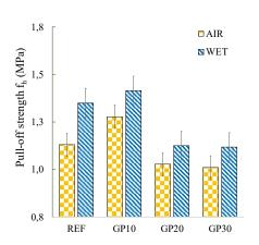
Fig.4 Average pull-off strength  $\mathbf{f}_{\mathbf{h}}$  of the subsurface layer.
