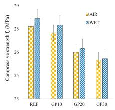
Fig.5 Average compressive strength f<sub>c</sub> of the subsurface layer.
